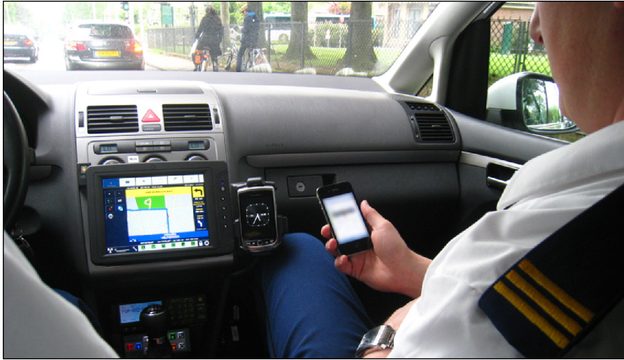
Figure 1.1. View on the cockpit of a police vehicle. Interior information processing tasks: operating the Mobile Data Terminal (MDT) and mobile phones, attending incoming radio messages, communication with the co-driver. Exterior information processing tasks: monitoring the environment, including other road users (i.e., as driver, and as police officer). NOTE: even though dedicated navigation technology has been developed (i.e., MDT), officers frequently make use of their mobile phones to find their way.
